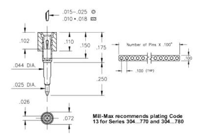
**Description:** Interconnect Socket Solderless Press-Fit Socket Accepts .015" - .025" (0,38 - 0,635 mm) dia leads
